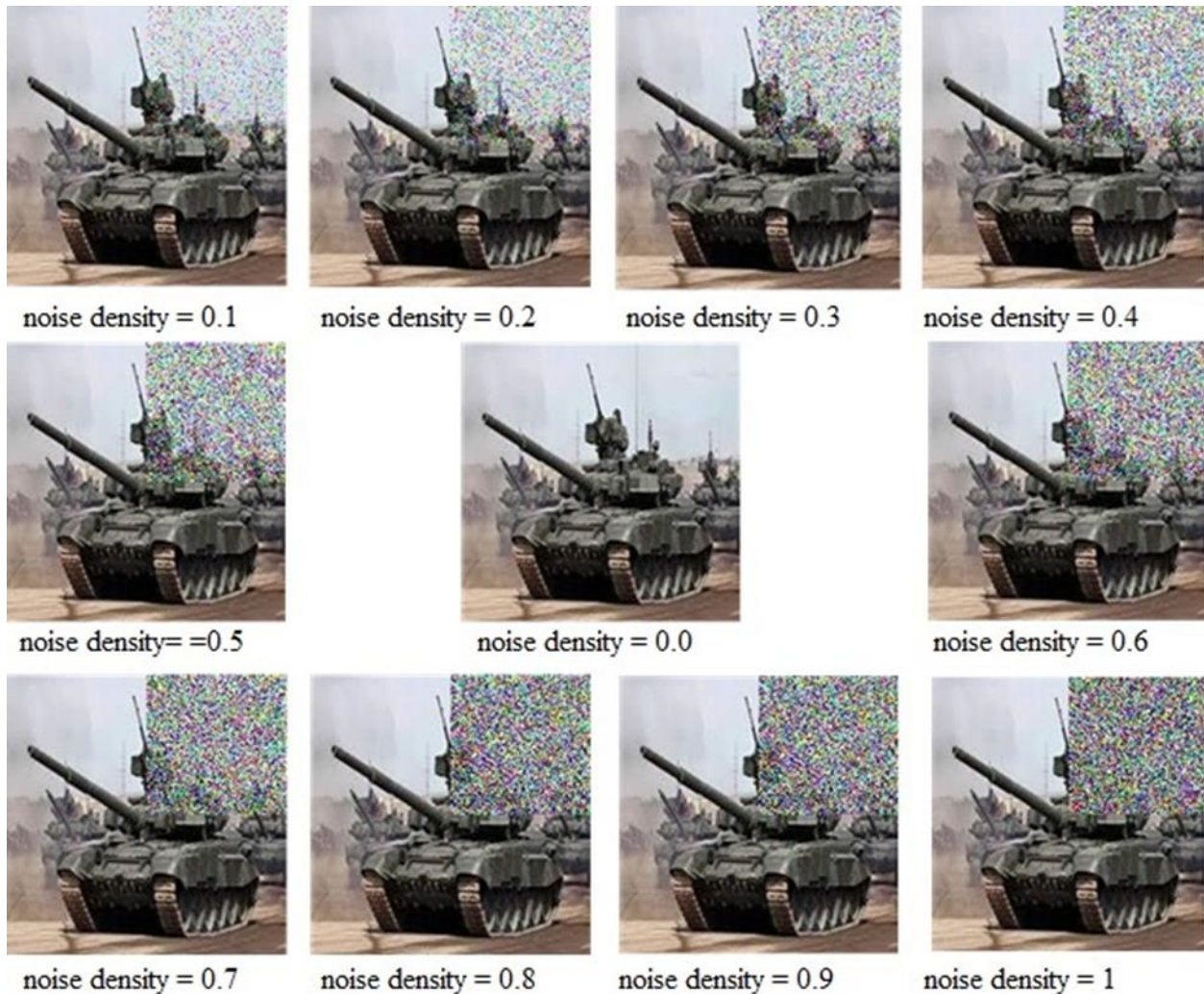
Fig. 4.16. Occlusion variants Quad2_TopRight for a "tank" class image implemented via the salt&pepper (impulse noise) function with different noise densities.
