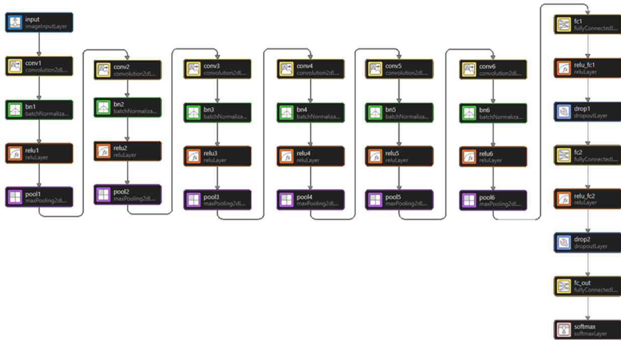
Fig. 4.9. Diagram of the implemented CNN with six convolutional blocks (without classification layer).
