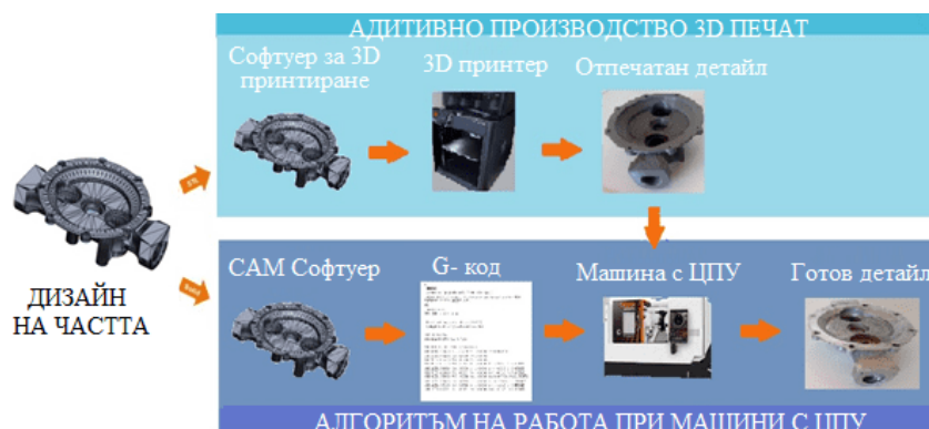
Fig. 4.7. Visualization of the technological algorithm for 3D printing and CNC machining.
