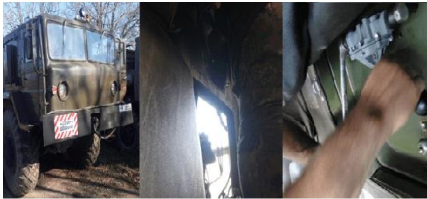
Fig. 4.5. Placing the restored PNM-1k samples on the fuel system of the MAZ-537G.
