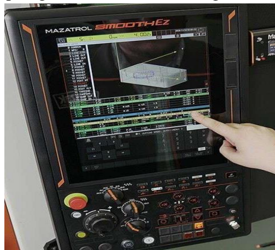
Fig. 3.9. CNC-centre MAZAK(Smooth technology) – setting parameters programmer.
