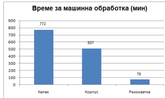
Fig. 4.10. CNC machining time of individual components of PNM-1k, manufactured using Mazak SmoothTech – from castings.
