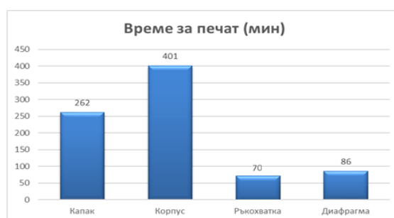
Fig. 4.8. Time for 3D printing of individual components of the PHM-1k, manufactured using FDM technology.
